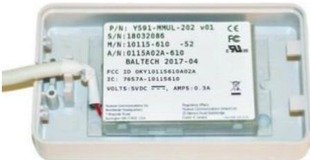
4. Fit the bottom plate on the top part of the housing, so that the loops engage the tabs.
