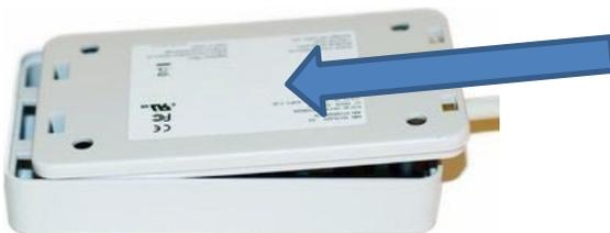
5. Press the cable end of the housing down until the parts snap together. No tools required.
