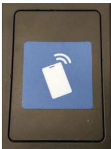
5. Snap the MFP cover shut, and install the "Place Card Here" sticker on the center of the cover.
