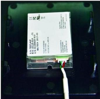
5. Connect the USB cable to the socket in the MFP and follow the manufacturer's instructions for reassembly.
