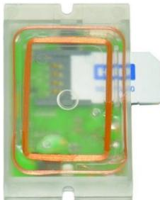
3. Use the edge of a coin or a flat-bladed screwdriver to push the SAM completely into the slot.
