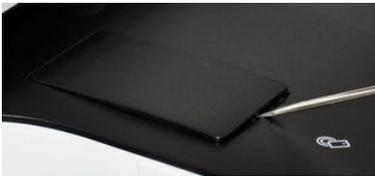
4. Connect the USB mini-B Plug to the socket in the MFP pocket, and place the reader in the pocket with the antenna (larger) side facing up.
